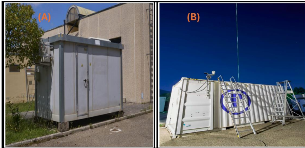
Figure 3.1. Aerosol lidar systems used in this study: (A) MUSA and (B) fixed Raymetrics operated at the CNR-IMAA Potenza station, and all systems are part of the ACTRIS/EARLINET networks and operate in multi-wavelength elastic-Raman configurations ( CIAO-CNR-IMAA Atmospheric Observatory, 2024 ).
