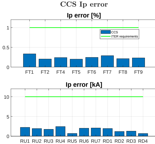
Figure 3.7: CCS plasma current reconstruction error with respect to the corresponding criteria.
