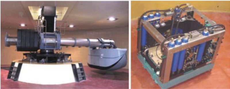
Figure 124. Left: IFSTTAR centrifuge; right: shear box (ACTIDYN actuator).
