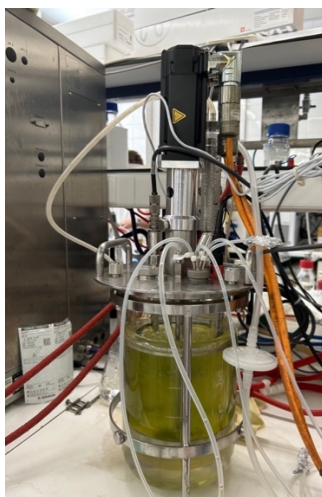
Figure 51. T. chuii cultivation in a 2-L bench-top bioreactor (Biostat B-plus Exclusive Flow, Sartorius Stedim, Germany) MixC.
