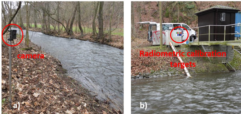
Figure 1.2: Installation of the camera (a) and the radiometric calibration panel (b) circled in red on the site of Meisdorf station.
