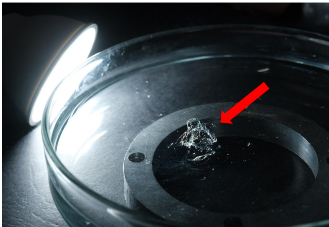
Figure 4.4. Picture of a free standing porous membrane suspended in diluted water.
