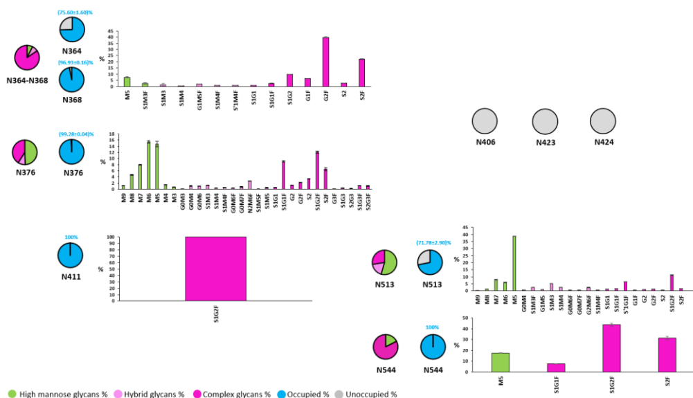
Figure 4.4. Site specific N -glycosylation profile of gB expressed in CHO cells (glycans relative abundancies and occupancies). The final output is given by the total average of the three average values. The detailed percentage values with their corresponding standard deviations are given in Tab. 4.1. The glycan structures with their corresponding names are given in Fig. 4.5.
