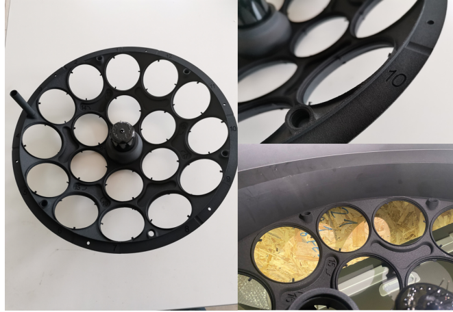
Figure 5.8: Details of the PMT support structure for the pouring of the optical gel and venting of air bubbles.
