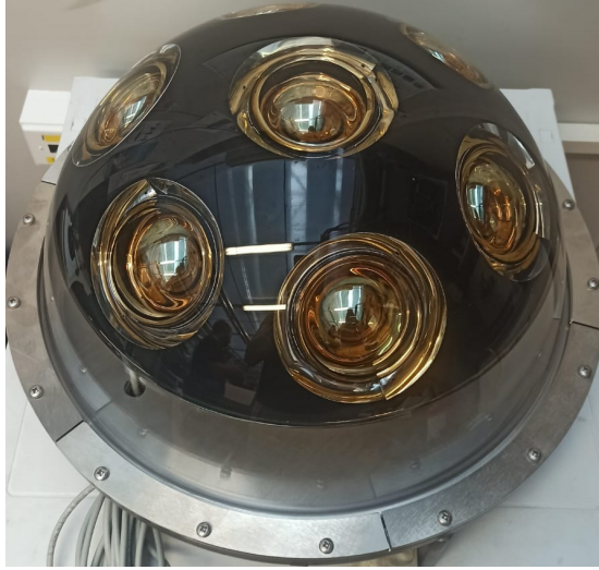
Figure 7.2: SWGO multiPMT prototype realized to do basic testing and characterization in lab.
