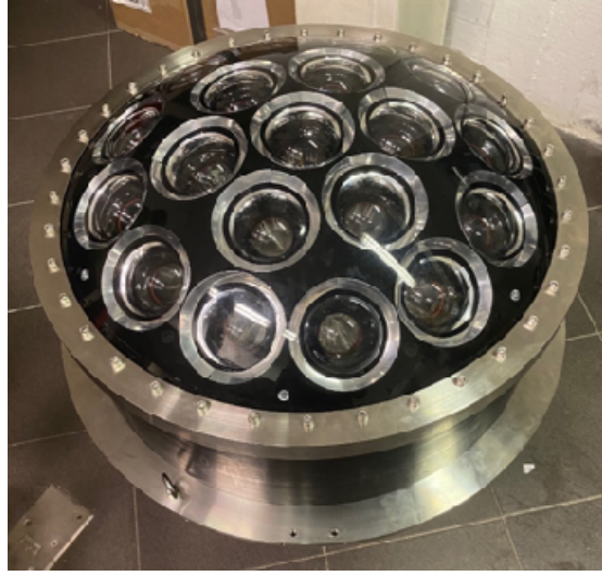
Figure 5.74: Picture of the first mPMT prototype assembled.
