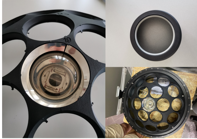
Figure 5.7: Details of the PMT support structure.
