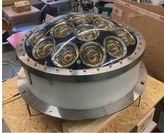
Figure 5.75: First fully operating mPMT assembled for Hyper-K.
