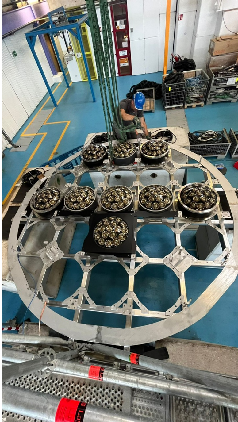
Figure 5.79: Overview of the bottom of the WCTE tank with the 4 mPMTs installed. They are clearly different by the IWCD ones, in particular is it possible to see the different backplate and clamping ring, much bigger in the Hyper-K ones.
