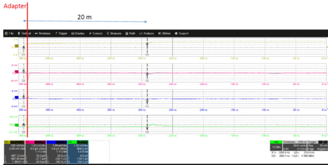
Figure 5.66: Standard CAT6 pulse test on the cable. The monitored lines on CH2, CH3 and CH4 shown no injection of the pulse.
