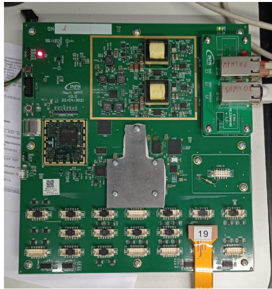
Figure 5.61: Thermal dissipation system of mPMT for testing. Top view.
