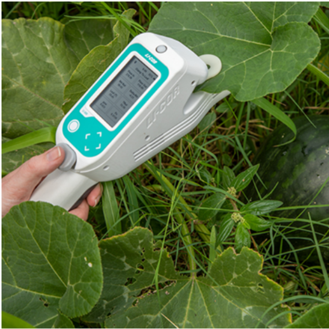
Figure 3.2. Data acquisition with LI-600 on pumpkin leaves.
