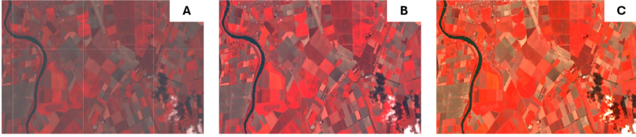
Figure 1.4. Raw S2 Product in DN (A), Top of Atmosphere (B), Bottom of Atmosphere (C).
