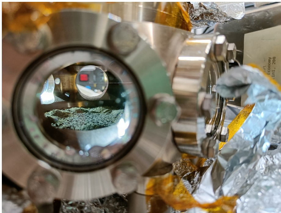
FIGURE 5.8: The sudden flow of hot air at 300 °C started a chemical reaction with the getter material (primarily zirconium) of the StarCell pump, inducing its complete burning out within a couple of minutes. The dust completely covered the bottom of the pumping chamber and contaminated most of the connections.
