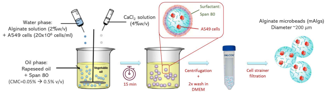
Figure 4.2: Representative scheme of fabrication route of A549 loaded mAlgs by external gelation method in a bulk emulsion.
