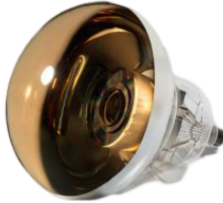
Figure 7.2: Hamamatsu 20" R12860-HQE PMTs.
