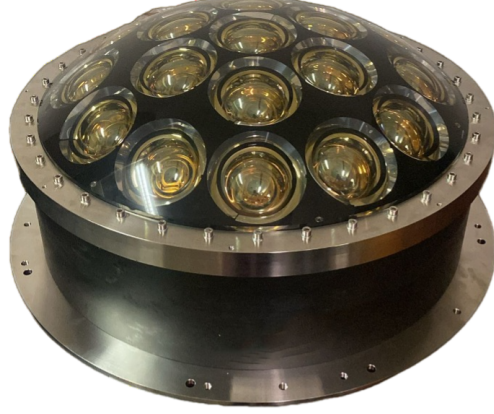
Figure 7.5: The final design of the mPMT prototype for Hyper-Kamiokande.
