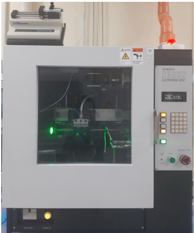
FIGURE 3.1: The electrospinning device used during the thesis work. This vertically aligned system facilitates the production of nanofiber matrices by transforming polymer solutions into fine fibers under high voltage.
