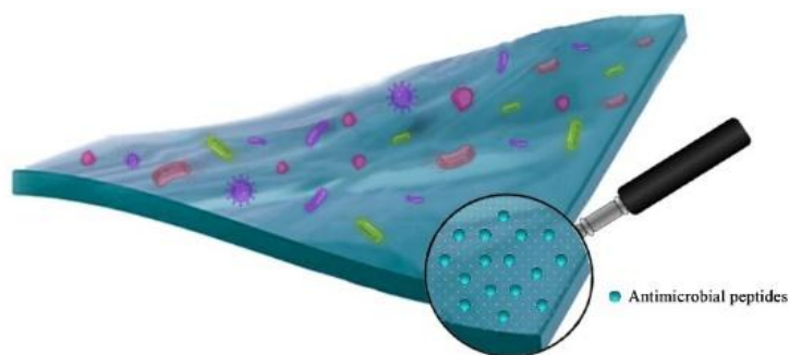
Fig. 1.1 Functionalized surface with antimicrobial peptides: cartoon representation of AMPs that actively target and neutralize microbial threats, including bacteria, viruses and fungi.
