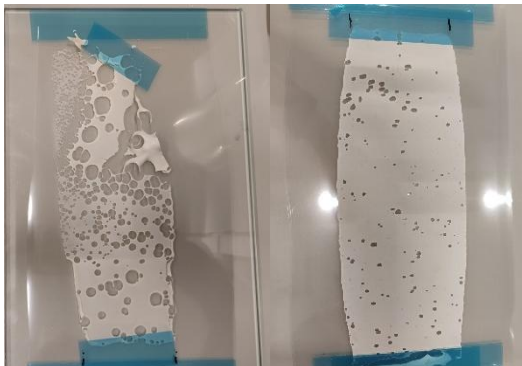
Fig. 2.13 Comparison of membranes produced with Synthesized Nylon 6,6 (left) and AMP3-Nylon (right).
