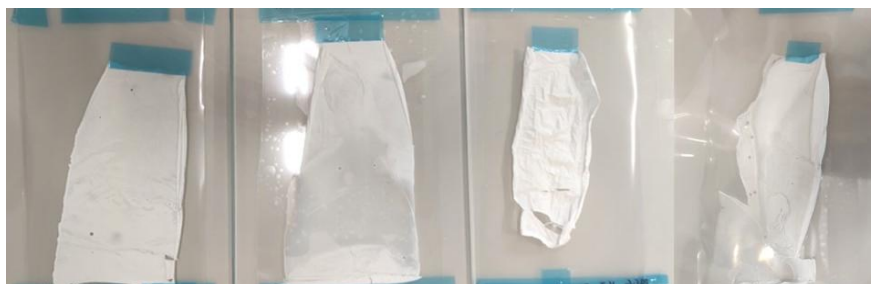
Fig. 2.11 Membranes prepared with increasing polymer concentrations, from left to right: 14, 16, 18, and 25% (w/w). The images illustrate the effect of polymer concentration on the structural integrity and morphology of the membranes, with higher concentrations leading to thicker and more stable structures.
