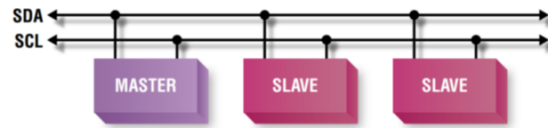
Figure 1.48: I 2 C protocol network showing master-slave communication over SDA and SCL lines (77)
