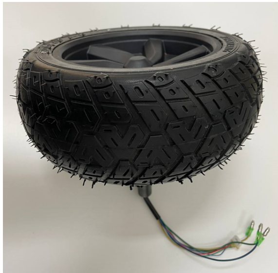
Figure A.24: DC motor-wheel subsystem used for propulsion in the Full-Scale Rover prototype
