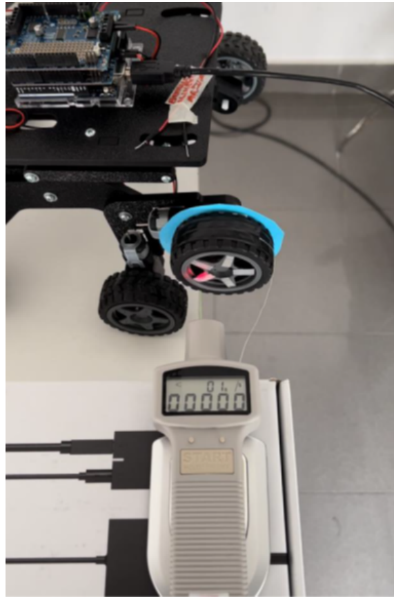
Figure 2.27: Electronic tachometer used to measure the rotational velocity of a wheel
