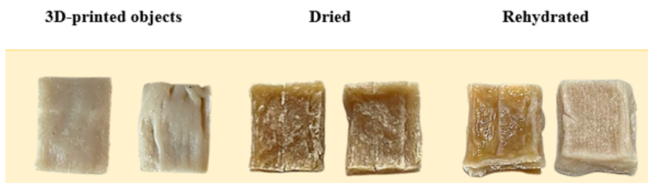
Figure 2.5. Macroscopic structure evolution of the 3D-printed samples (cold-extruded on the left and hot-extruded on the right of each column) from left to right: 3D-printed objects; dried samples at 60^{\circ}\text{C} for 6 h; rehydrated objects for 1 h in lukewarm water.
