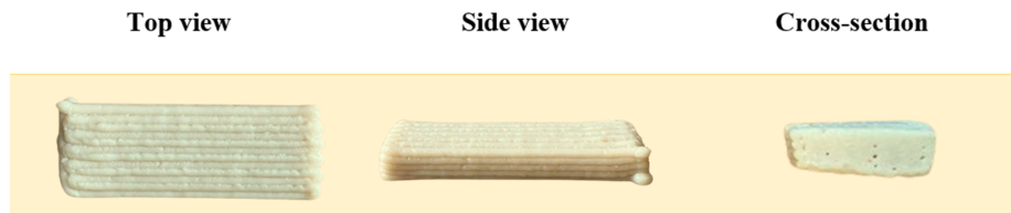
Figure 2.3. From left to right: 3D-printed object top view, side view and cross-section. CAD dimensions: 40 mm \times 15 mm \times 6 mm.
