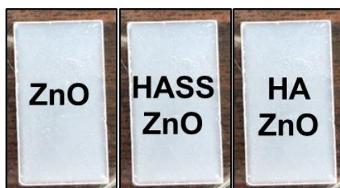
Figure 3.19. Glass supports with nanostructured films of ZnO, HASS-doped/ZnO and HA-doped/ZnO nanocatalysts.
