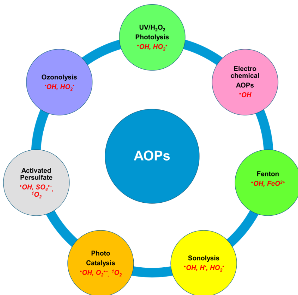
Figure 2.22. Classifications of AOP-based technologies and the ROS involved.
