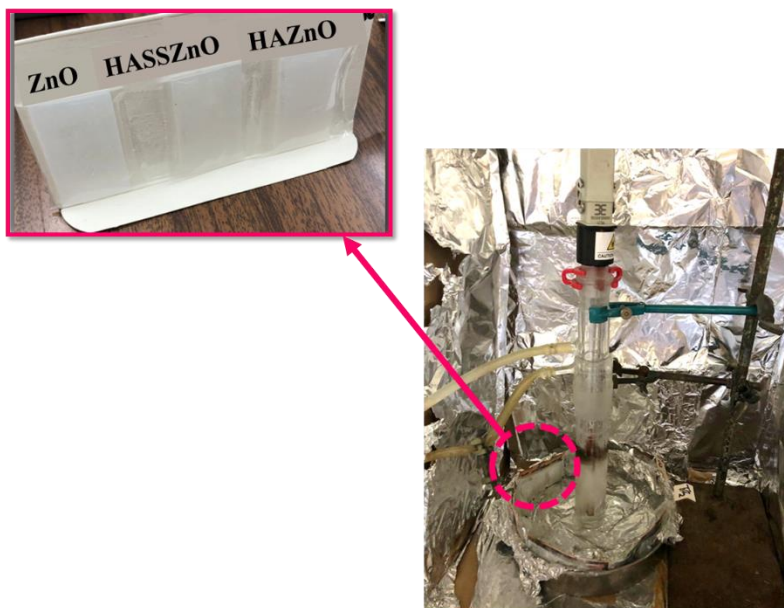
Figure 3.20. Photodegradation tests of LLDPE and PLA slices deposited on glass supports in a bath containing water and exposed to UVA lamp.
