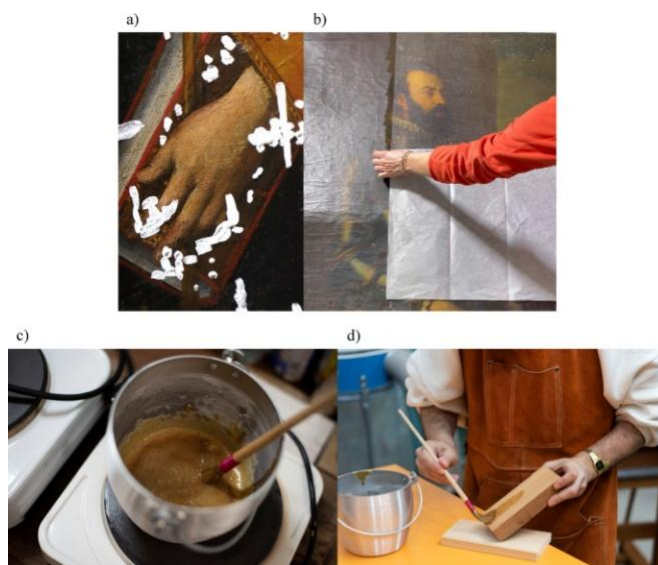
Figure 1. (a) Plastering with rabbit glue and Bologna gypsum, “Sacred conversation with the Madonna of the girdle”, Unknown, fifteenth century, panel painting, church of SS. Annunziata—Sorrento (NA); (b) Facing with rabbit glue, “portrait of a warrior”, Unknown, seventeenth century, canvas painting, private collection; (c) preparation of BM5 glue samples; (d) use of BM5 glue in carpentry.
