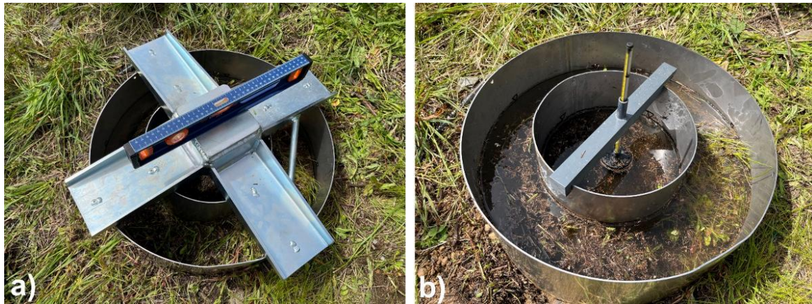
Figure A1.4 – Double ring infiltrometer test: a) placement of the two concentric rings; b) initial condition in which both rings are simultaneously filled, maintaining the same water level.
