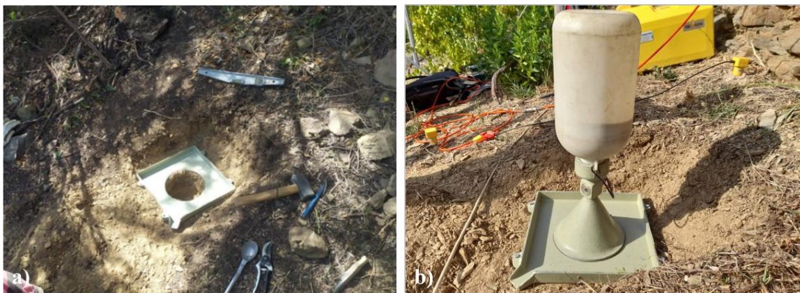
Figure A1.3 - Soil density tests: a) hole excavated for the test; b) sand cone used for field analyses
