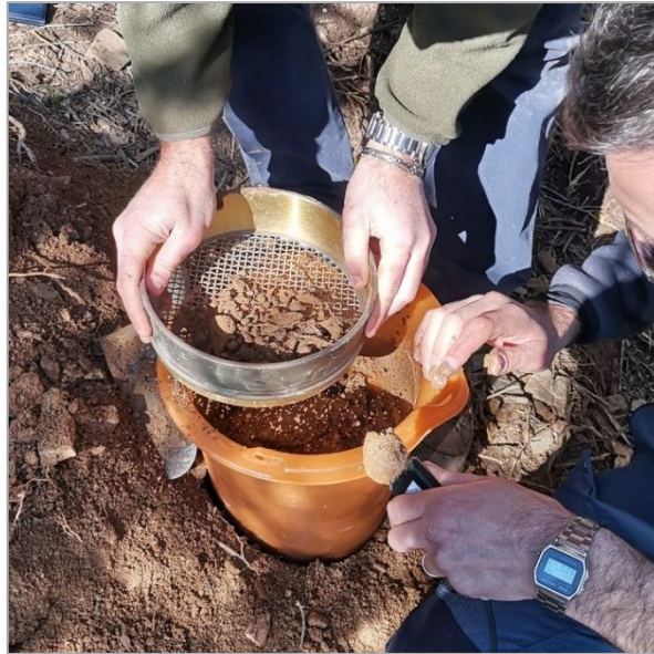
Figure 3.12 - Preparation of a fine material and water slurry which was packed around the TEROS21 sensor.
