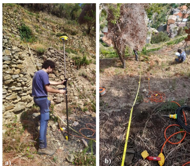
Figure A1.1 - On the left, GNSS surveys for the acquisition of the array geometry. On the right, the arrangement of geophones (connected to the seismograph via cables) along a longitudinal seismic alignment.
