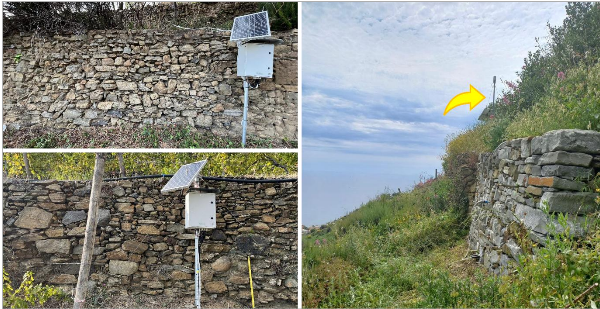
Figure 3.14 - Multiparametric monitoring systems and dataloggers installed at each monitoring site.
