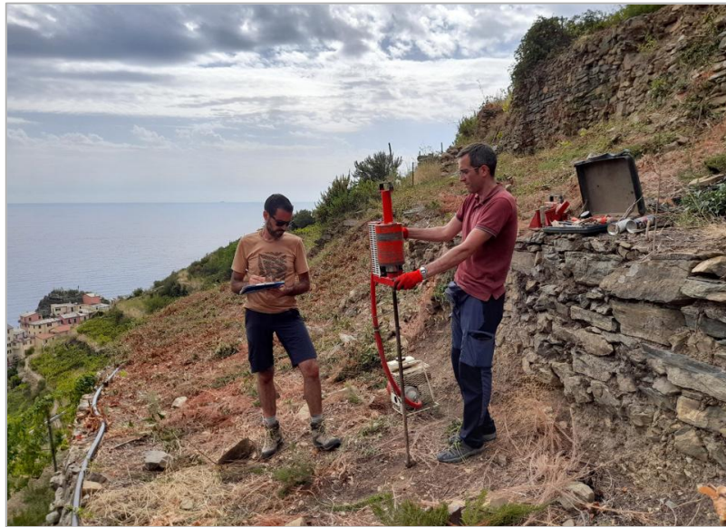
Figure A1.2 - Dynamic probing test execution.
